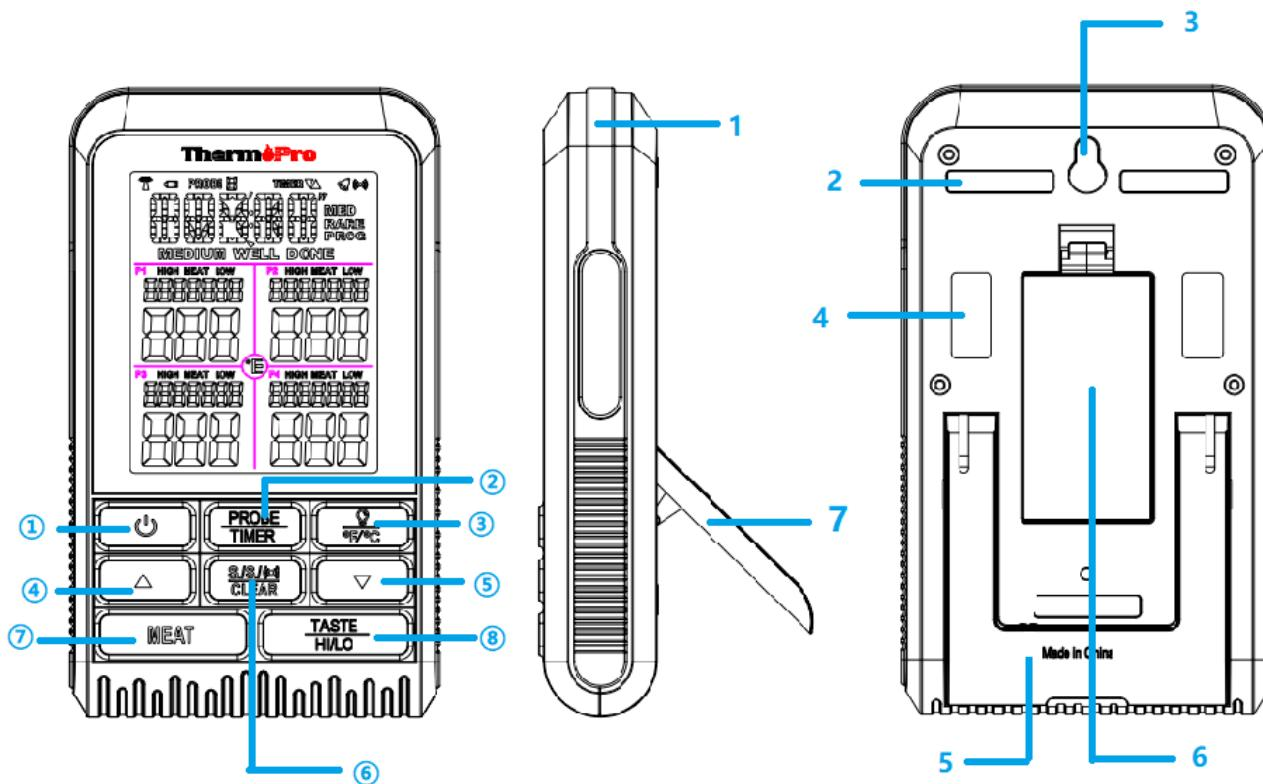
1 Soft Rubber Sleeve 2Anti-slip 3Hanging Hole 4 Magnet 5 Flip-out Counter Top Stand 6 Battery Compartment 7 Tabletop Stand
