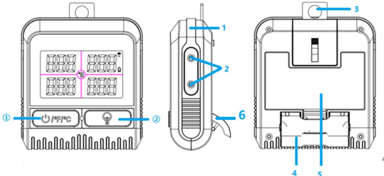
1 Soft Rubber Sleeve 2 Probe Sockets 3 Hanging 4 Flip-out Counter Top Stand 5 Battery Compartment 6 Tabletop Stand
