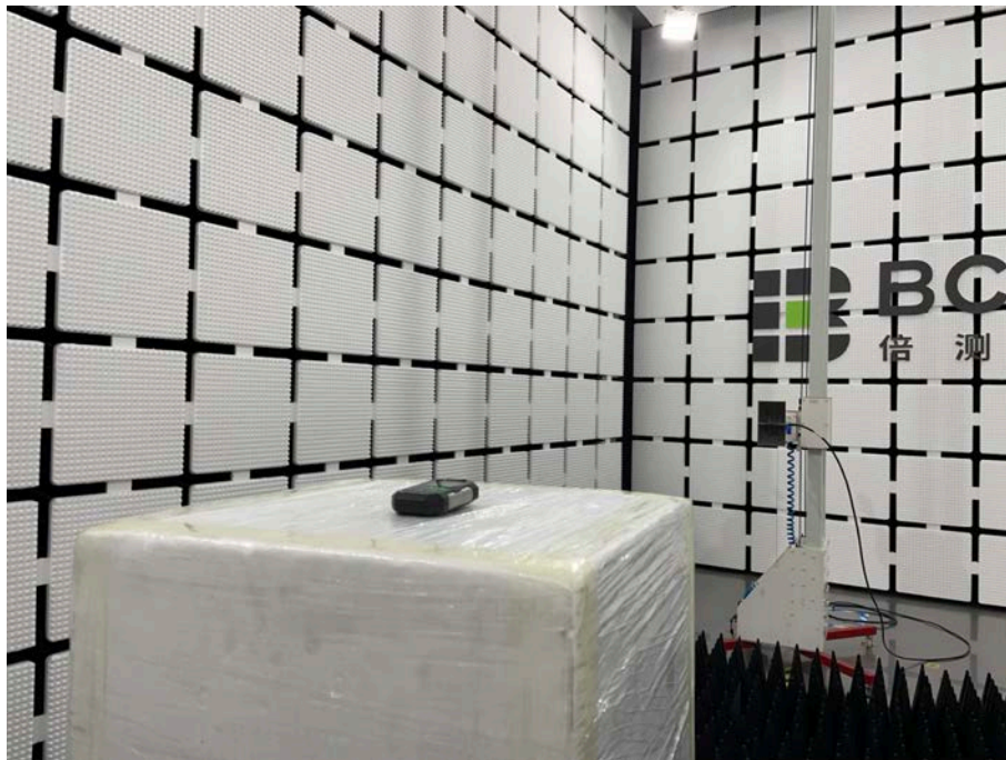
Spurious Emission Test Setup (Above 1GHz)
