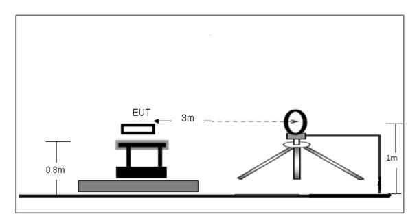
(B) Radiated Emission Test-Up Frequency 30MHz~1GHz
