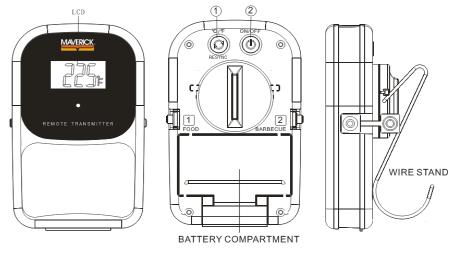
• LCD (Liquid Crystal Display) – displays temperature of both FOOD and BARBECUE. It will automatically switch between FOOD and BARBECUE displays.
