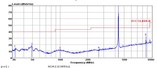
Reading CabLos Antfac Measured Limit Over MHz dBuV  $^{\mathrm{dB}}$ dB/m dBuV/m dBuV/m dВ 32.07 0.37 2.40 12.32 15.09 40.00 -24.91 OP 49.01 4.97 0.35 13.31 18.63 40.00 -21.37 QP 99.88 -1.29 0.60 13.15 12.46 43.50 -31.04 QP 264.75 -0.27 1.03 12.20 12.96 46.00 -33.04 QP 434.07 87.81 Peak 6 868.14 10.66 1.87 20.77 33.30 46.00 -12.70 Peak
