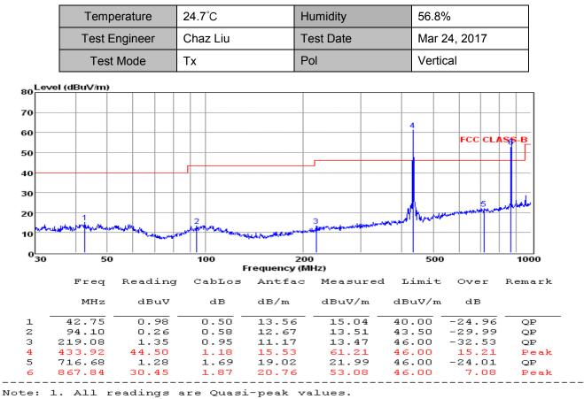
2. Measured= Reading + Antenna Factor + Cable Loss
