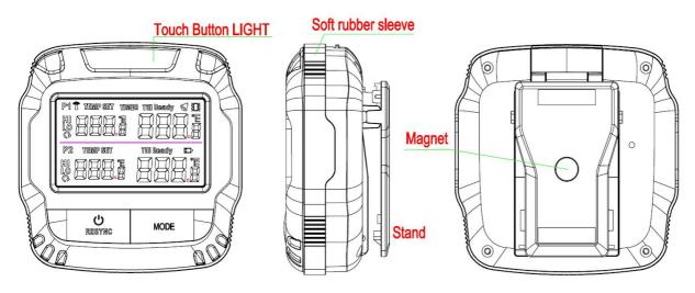
1.LCD (Liquid Crystal Display) – Displays all icons, temperature
