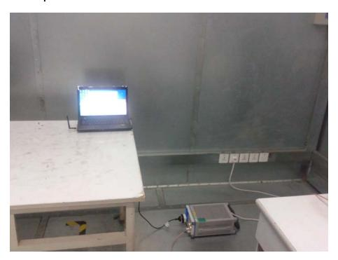
Set-up for Radiated Emission Test
