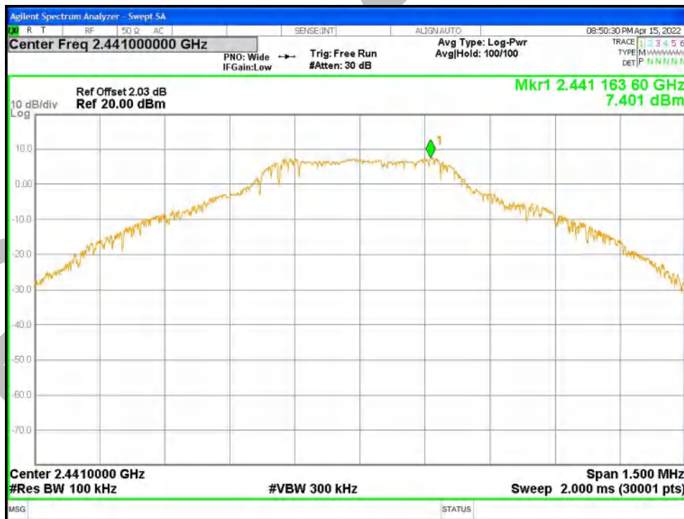
Tx. Spurious NVNT 1-DH1 2441MHz Ant1 Emission
