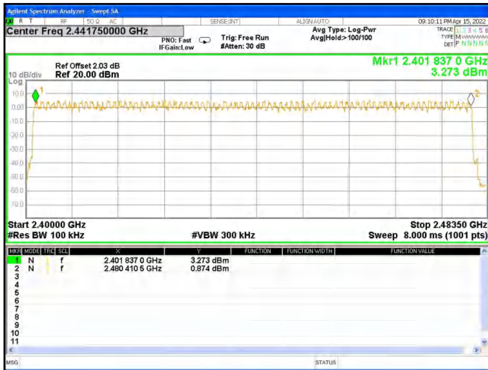
Hopping No. NVNT 3-DH1 2441MHz Ant1
