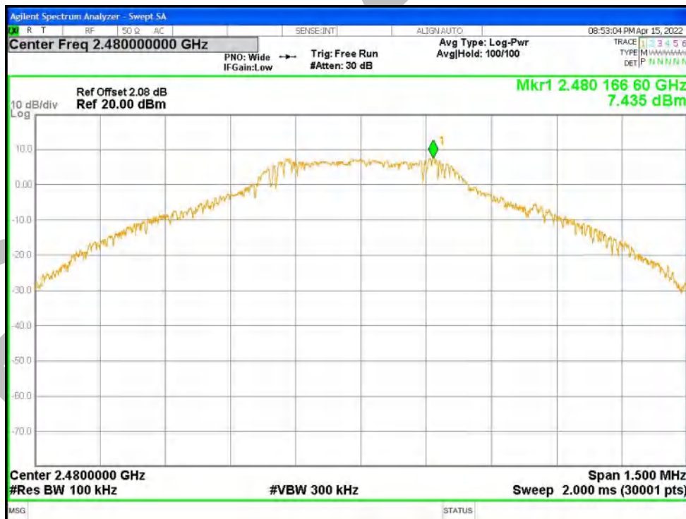
Tx. Spurious NVNT 1-DH1 2480MHz Ant1 Emission
