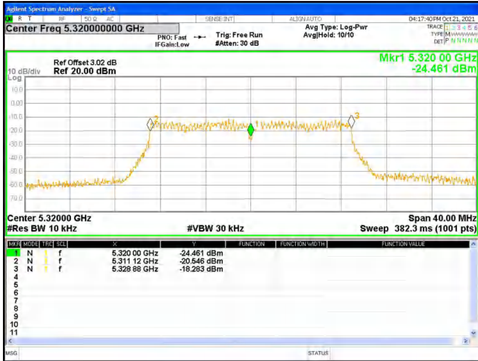
Freq. Stability NVNT ac20 5500MHz Ant1
