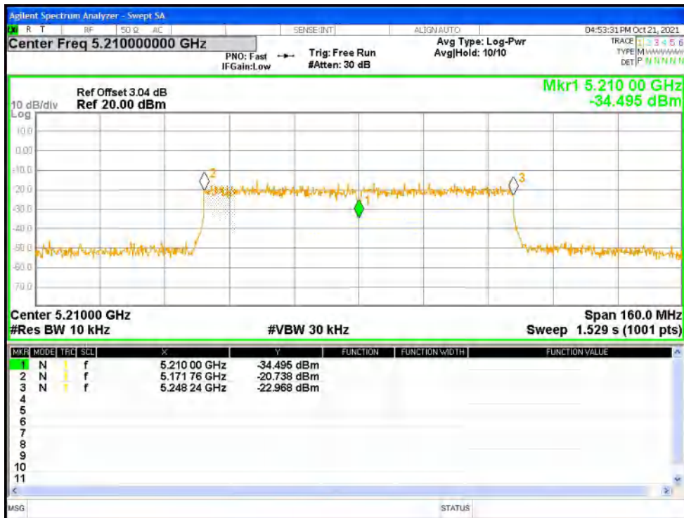
Freq. Stability NVNT ac80 5290MHz Ant1
