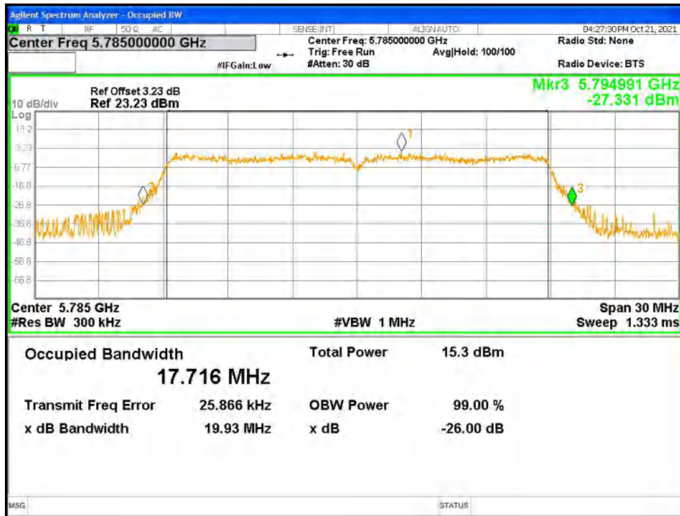
-26dB Bandwidth NVNT ac20 5825MHz Ant1
