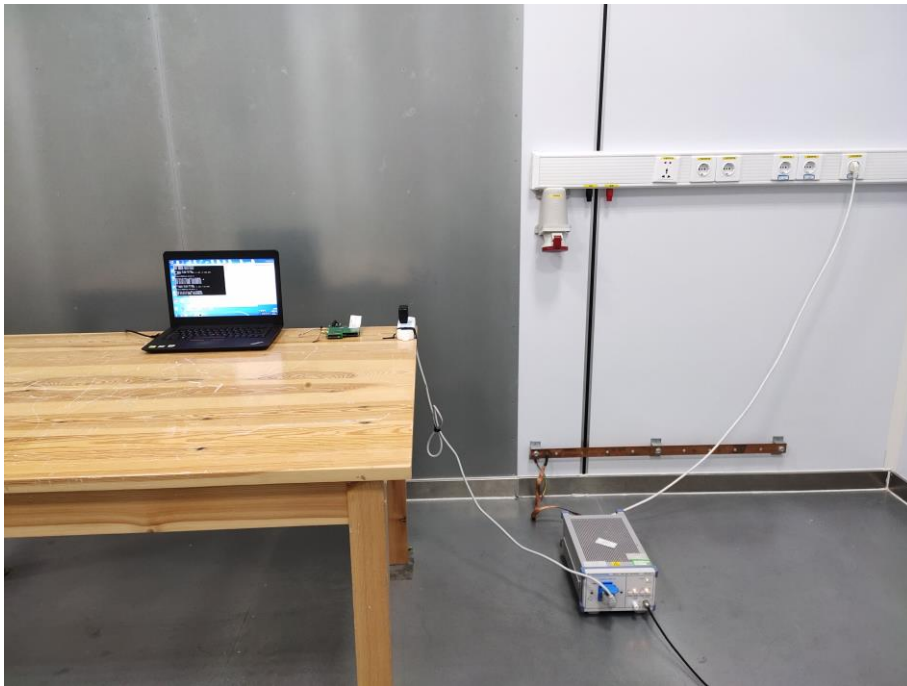
Fig. 4 Power line conducted emission setup photo
