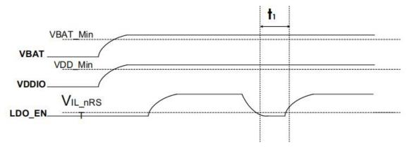
Figure 5: Reset Timing
