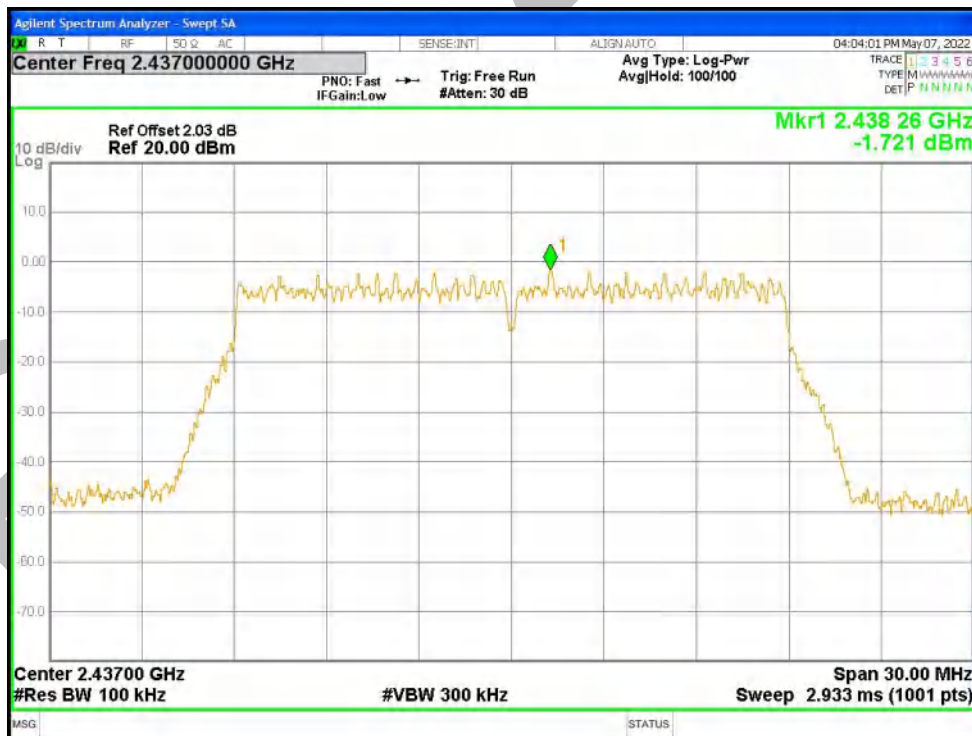
Tx. Spurious NVNT n20 2437MHz Ant1 Emission
