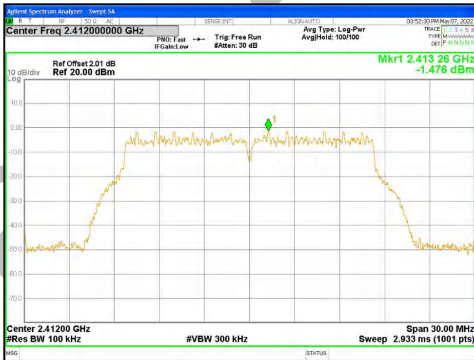
Band Edge NVNT g 2412MHz Ant1 Emission
