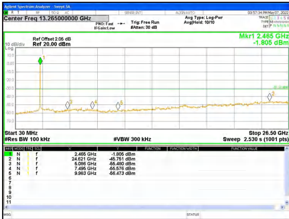
Tx. Spurious NVNT n20 2412MHz Ant1 Ref
