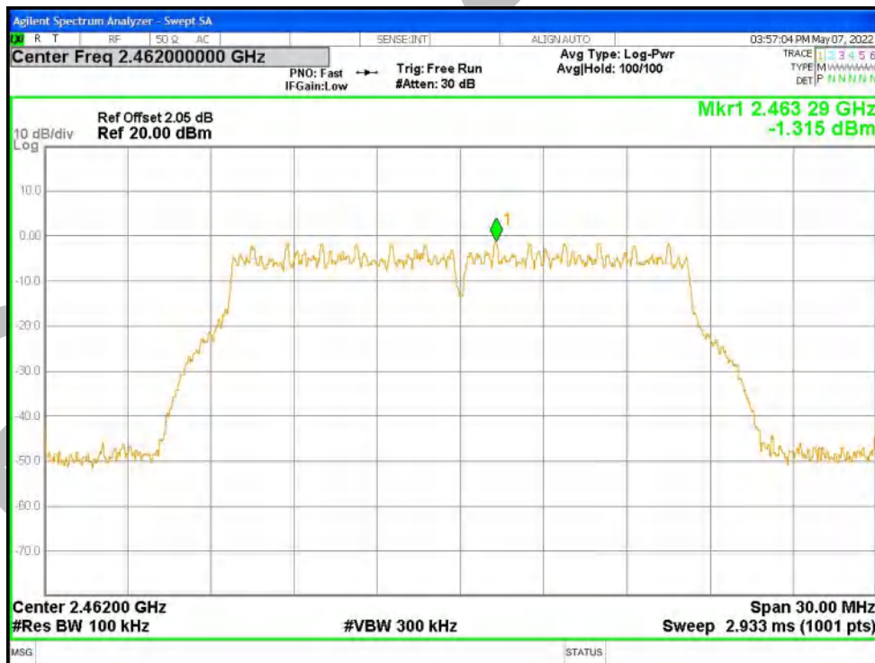
Tx. Spurious NVNT g 2462MHz Ant1 Emission
