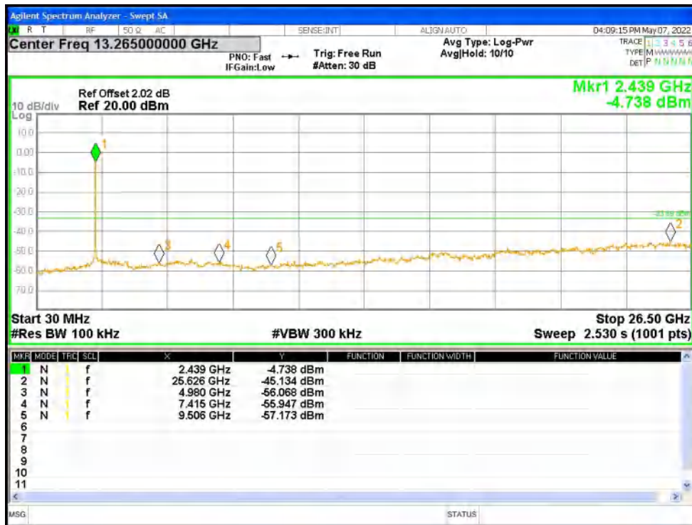
Tx. Spurious NVNT n40 2437MHz Ant1 Ref
