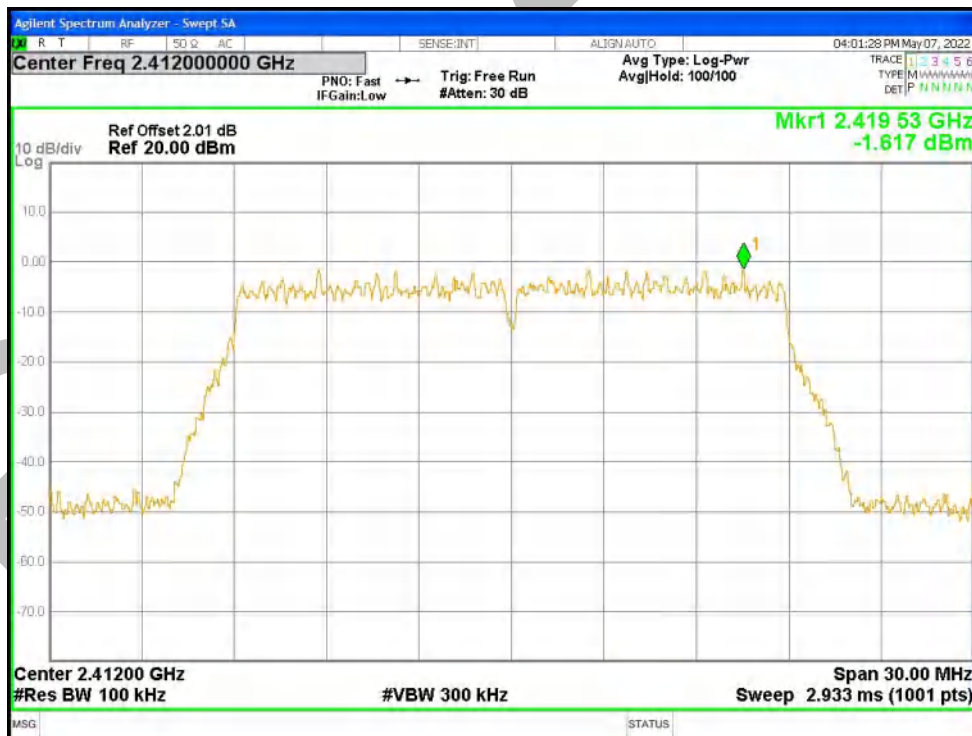
Band Edge NVNT n20 2412MHz Ant1 Emission
