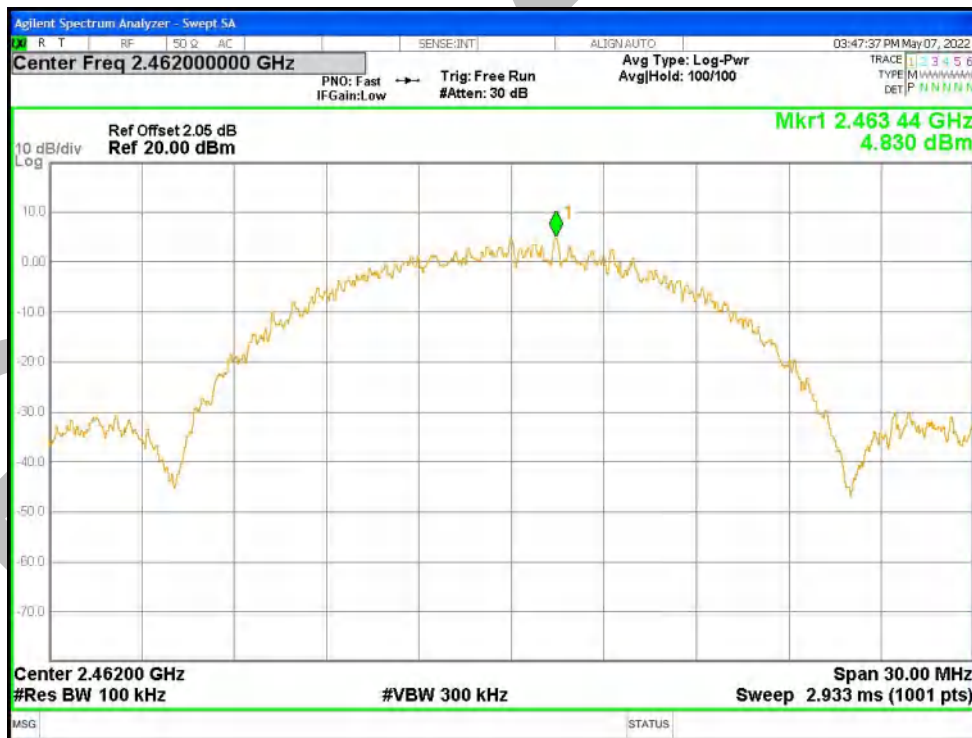
Tx. Spurious NVNT b 2462MHz Ant1 Emission
