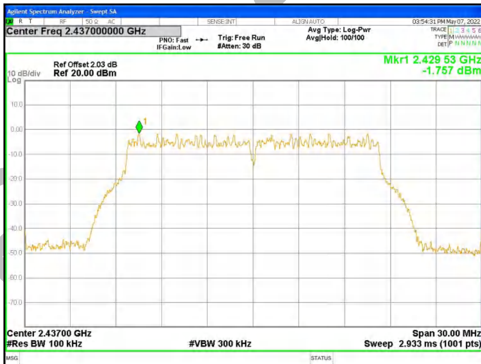
Tx. Spurious NVNT g 2437MHz Ant1 Emission
