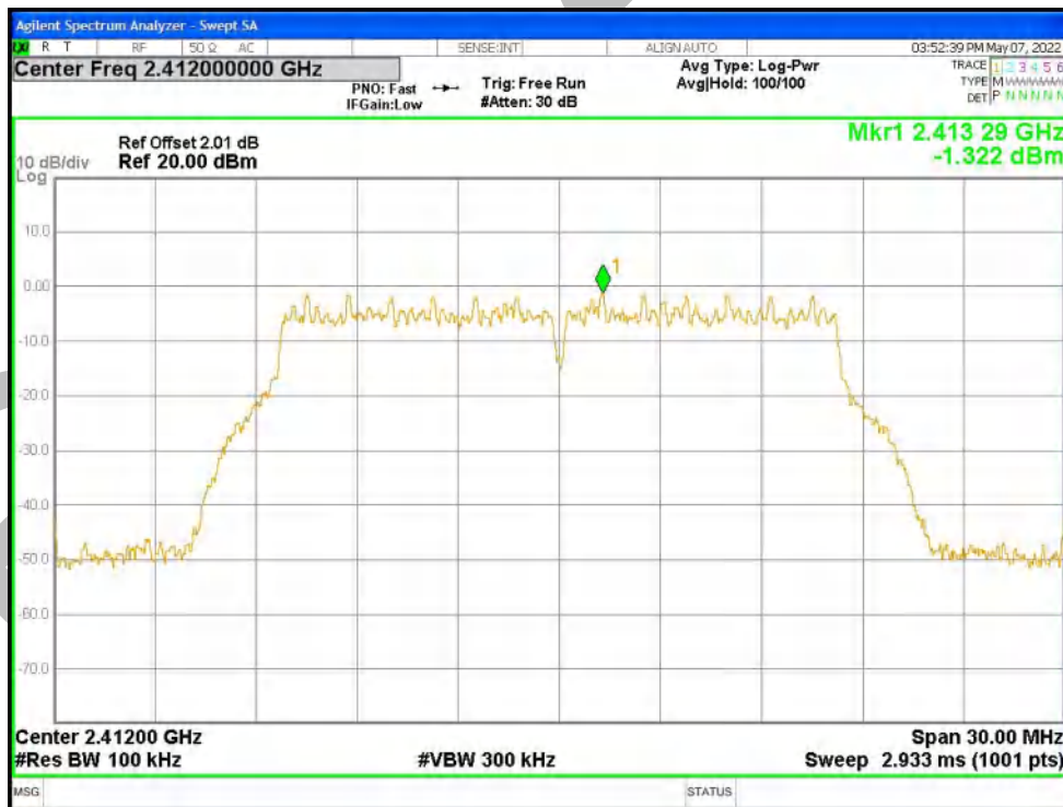
Tx. Spurious NVNT g 2412MHz Ant1 Emission
