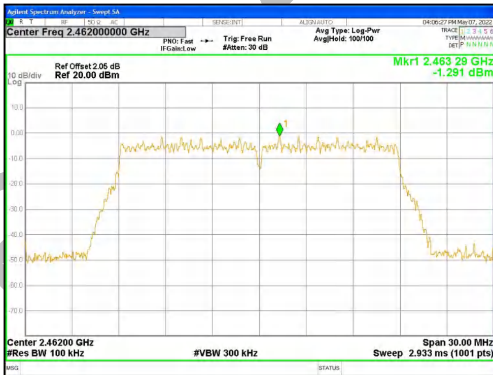
Tx. Spurious NVNT n20 2462MHz Ant1 Emission
