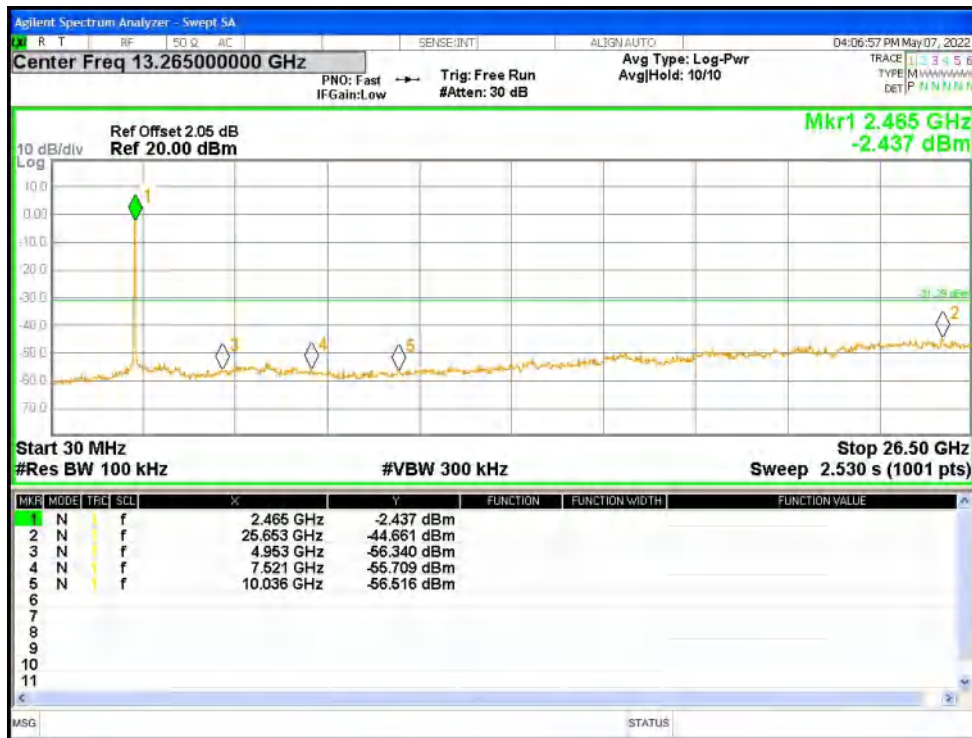
Tx. Spurious NVNT n40 2422MHz Ant1 Ref
