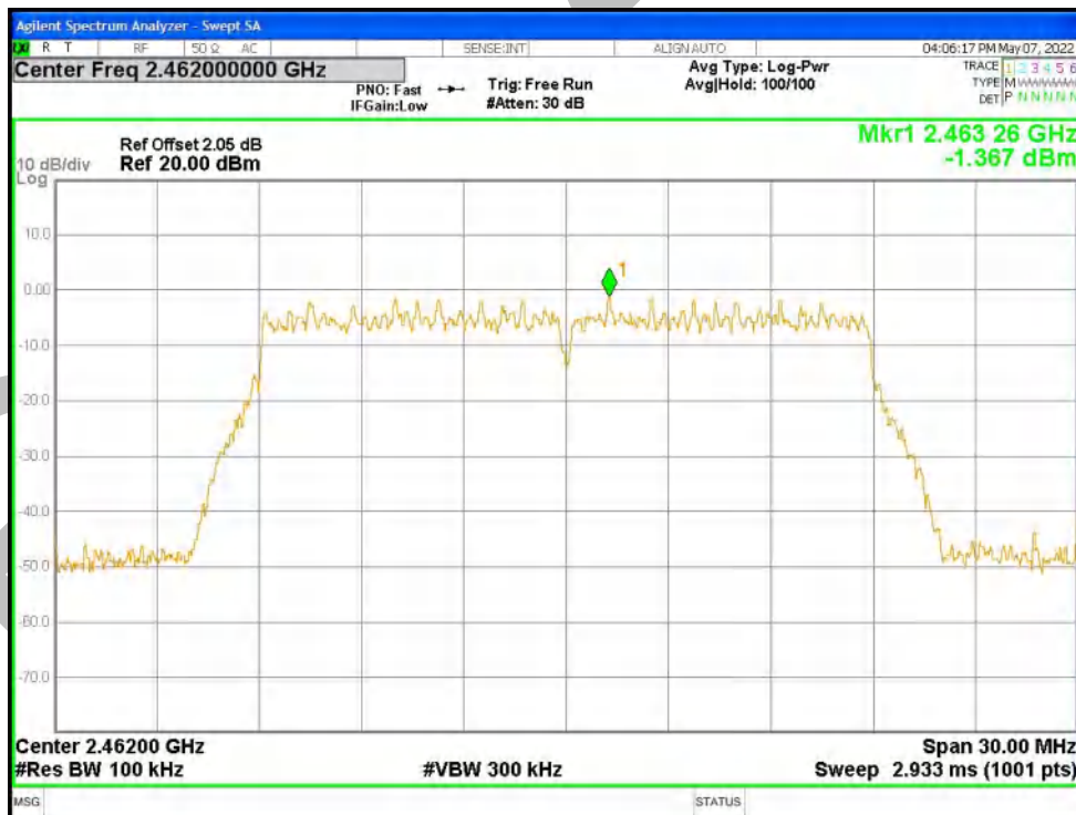
Band Edge NVNT n20 2462MHz Ant1 Emission
