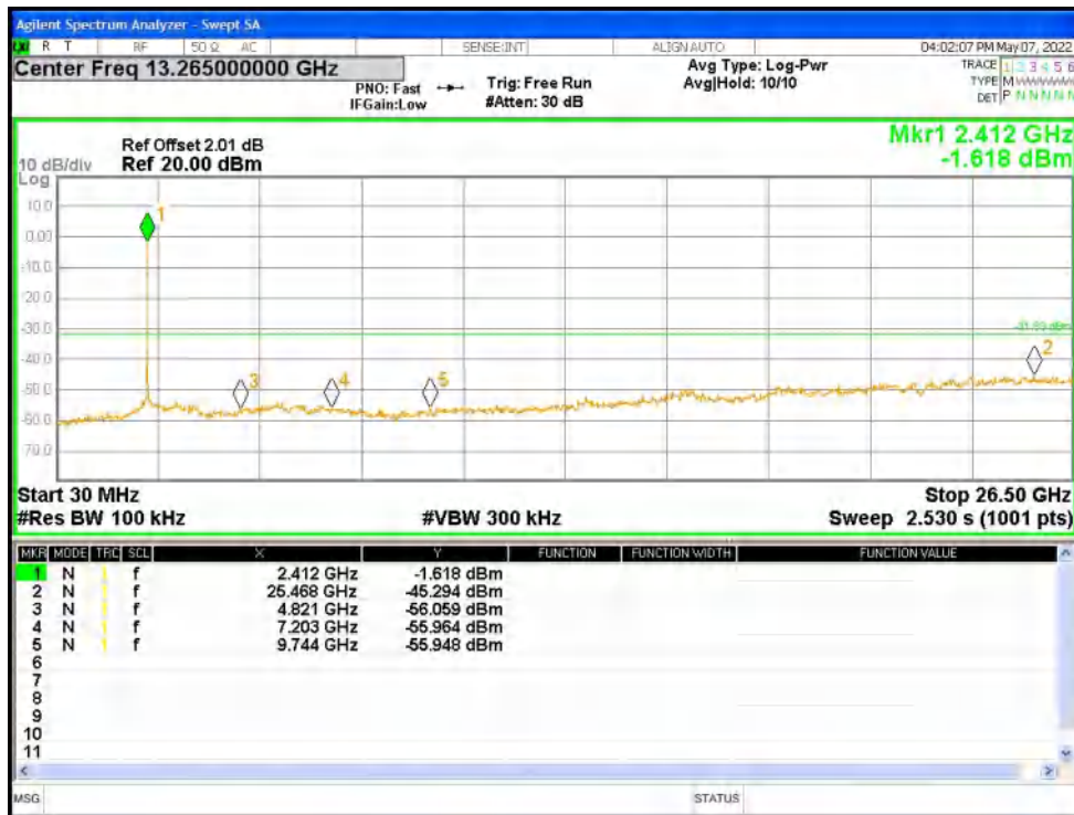
Tx. Spurious NVNT n20 2437MHz Ant1 Ref
