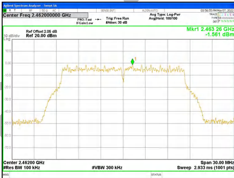
Band Edge NVNT g 2462MHz Ant1 Emission
