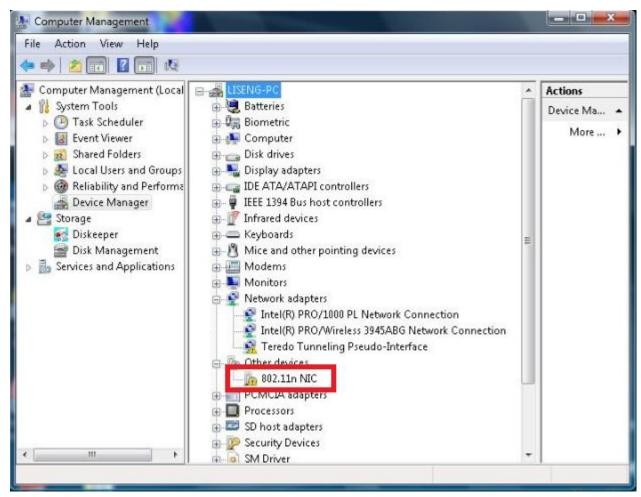
2. Copy the corresponding driver "RTLWlanU\_WindowsDriver\_1019.0.0518.2012\_UI\_1.00.0191\_EU" into the PC, and install driver, the installation methods: open the file "RTLWlanU\_WindowsDriver\_1019.0.0518.2012\_UI\_1.00.0191\_EU", double click "Setup" installation program, guide to install.
