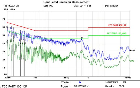
Limit: FCC PART 15C\_QP EUT: WIFI+BT Module M/N: 8223A-SR Mode: TX(BLE)
