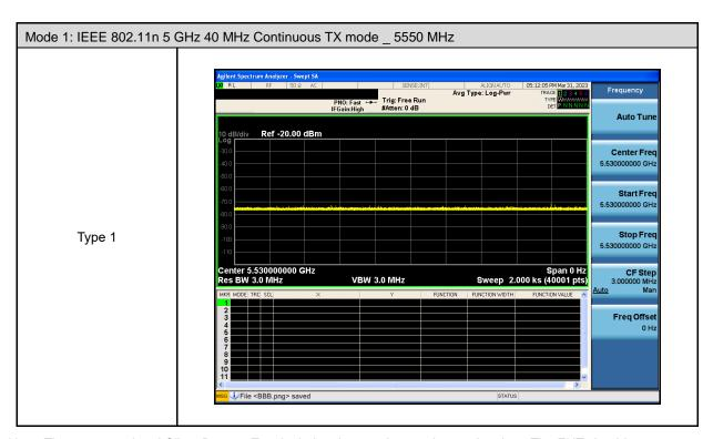
Note: The non-associated Client Beacon Test is during the 30 minutes observation time. The EUT should not make any transmissions in the DFS band after EUT power up.
