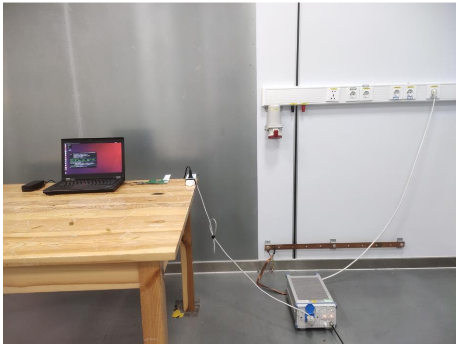
Fig. 4 Power line conducted emission setup photo
