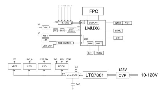
The i.MX 6ULL is a power efficient and cost-optimized applications processor family featuring an advanced implementation of a single Arm Cortex-A7 core, which operates at speeds up to 900 MHz.
