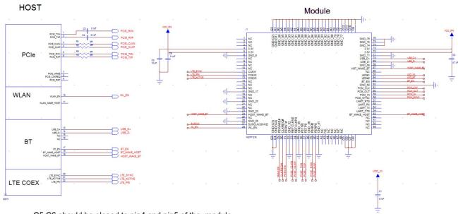
C5 C6 should be closed to pin4 and pin5 of the module
