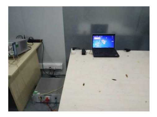
Radiation Emission Test Setup (Below 30MHz)
