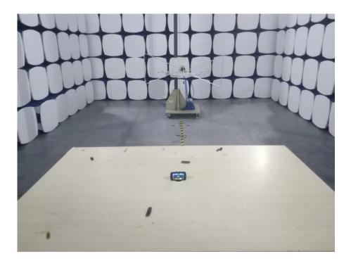
Radiation Emission Test Setup (1GHz to 18GHz)
