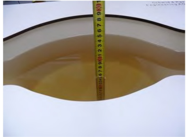
Liquid depth in the body phantom (835MHz)
