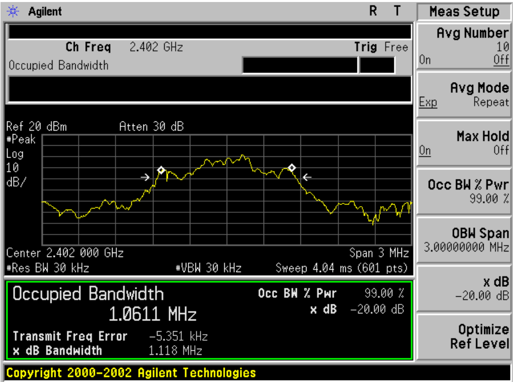
TEST PLOT OF BANDWIDTH FOR LOW CHANNEL
