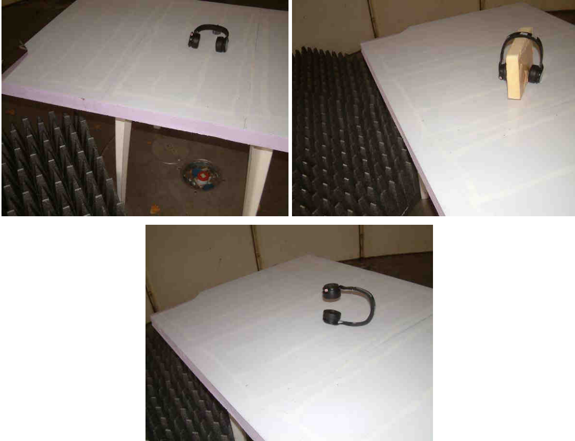
Photo of test setup for Radiated Disturbance
