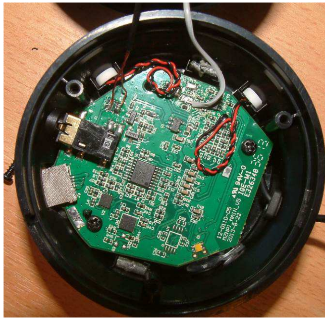
Internal view of cup (Speaker 2 removed, main PCB)
