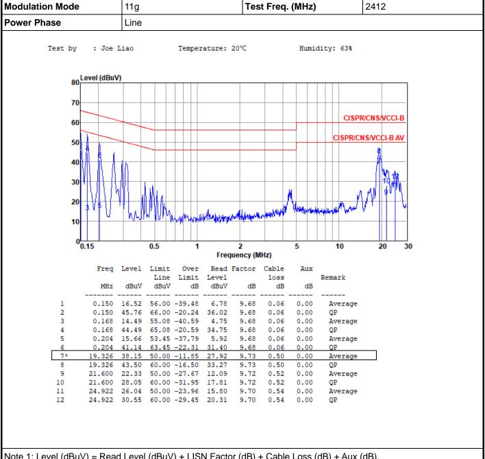
Note 1: Level (dBuV) = Read Level (dBuV) + LISN Factor (dB) + Cable Loss (dB) + Aux (dB).
