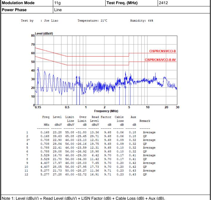
Note 1. Level (dBuv) = Read Level (dBuv) + Lish Factor (dB) + Cable Loss (dB) + Aux (dB).
