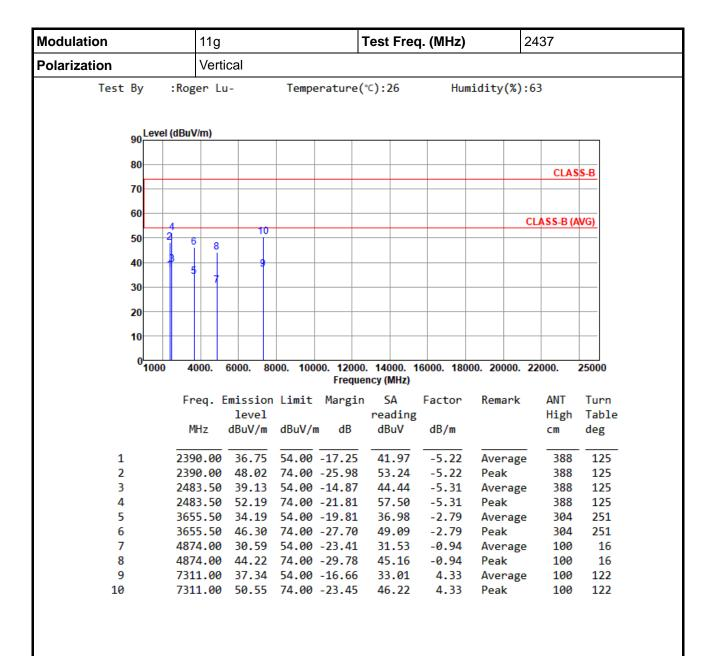
\*Factor includes antenna factor, cable loss and amplifier gain
