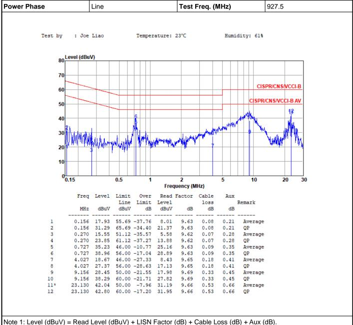
2: Over Limit (dB) = Level (dBuV) - Limit Line (dBuV).
