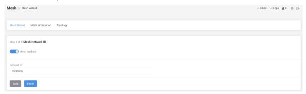
Network ID – an unique ID for adding RE into existing mesh connection
