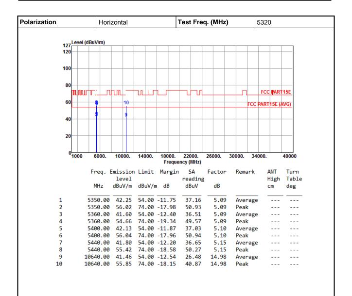
Note 1: ">20dB" means spurious emission levels that exceed the level of 20 dB below the applicable limit. Note 2: For restricted bands, the peak measurement is fully sufficient, as the max field strength as measured with the Peak-Detector meets the AV-Limit so that the AV level does not need to be reported in addition.
