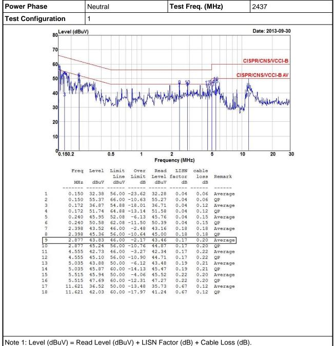
Note 1: Level (dBuV) = Read Level (dBuV) + LISN Factor (dB) + Cable Loss (dB). 2: Over Limit (dBuV) = Level (dBuV) - Limit Line (dBuV).
