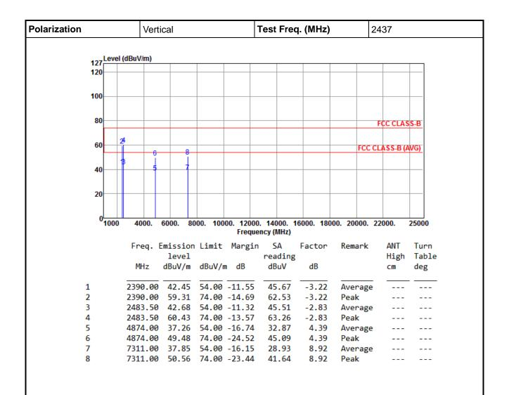
Note 3: For un-restricted bands, unwanted emissions shall be attenuated by at least 20 dB relative to the maximum measured in-band level.
