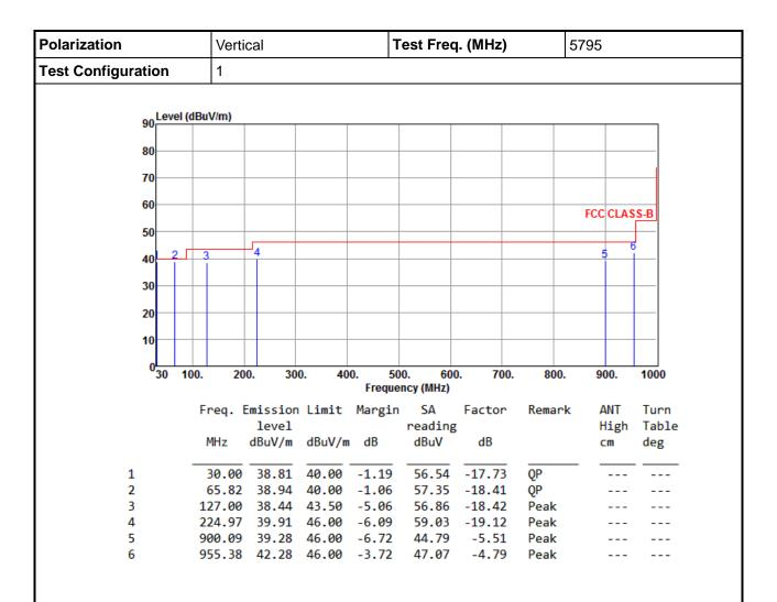
Note 1: Emission Level (dBuV/m) = SA Reading (dBuV/m) + Factor\* (dB) \*Factor includes antenna factor, cable loss and amplifier gain Note 2: Margin (dB) = Emission level (dBuV/m) – Limit (dBuV/m).
