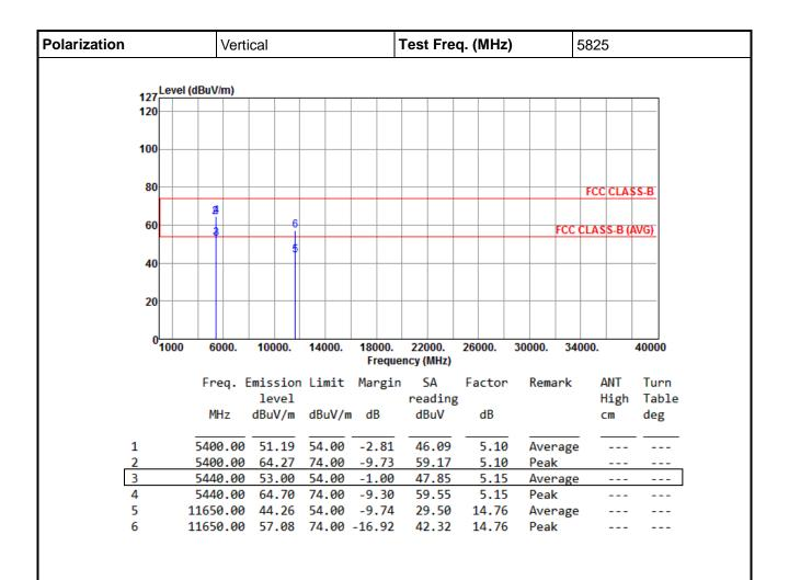
Note 3: For un-restricted bands, unwanted emissions shall be attenuated by at least 20 dB relative to the maximum measured in-band level.
