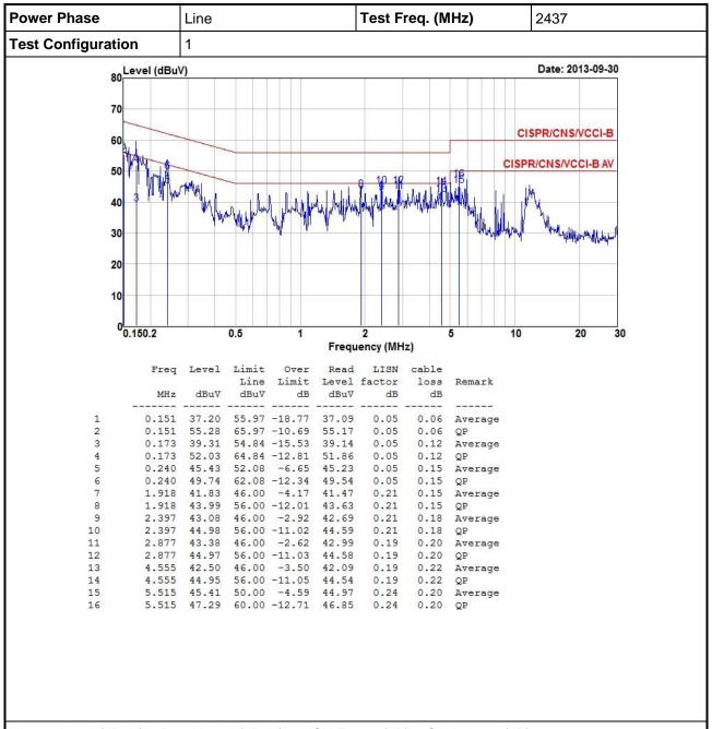
Note 1: Level (dBuV) = Read Level (dBuV) + LISN Factor (dB) + Cable Loss (dB).
