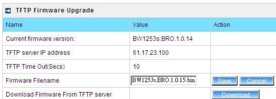
Figure 121 – TFTP Firmware Upgrade setting
