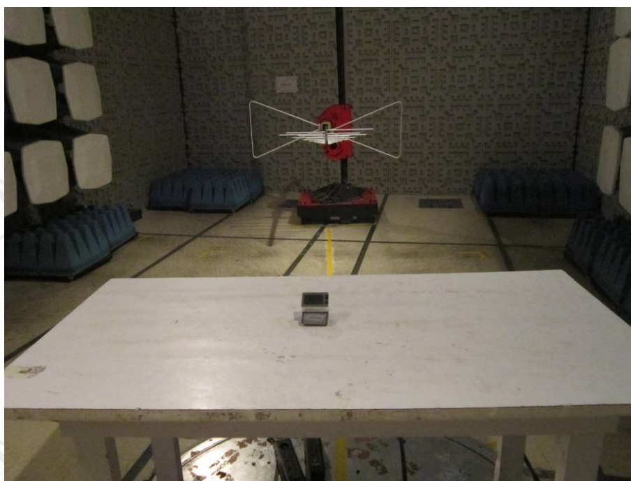
TEST SETUP OF RADIATED EMISSION-2
