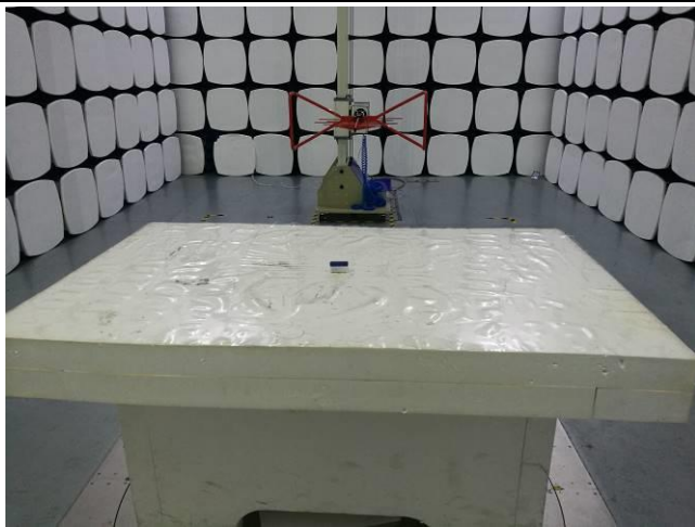
Radiated Spurious Emissions Test Setup Below 1GHz
