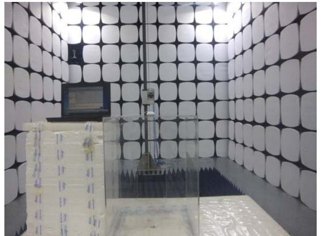
Radiated Spurious Emissions Test Setup Above 1GHz
