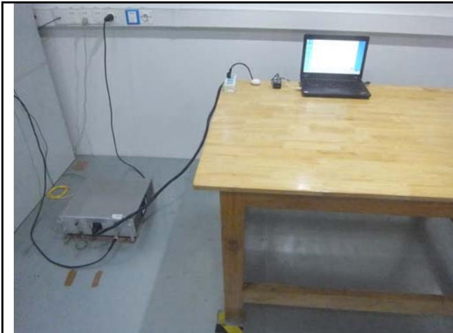
Conducted Emissions Test Setup Front View
