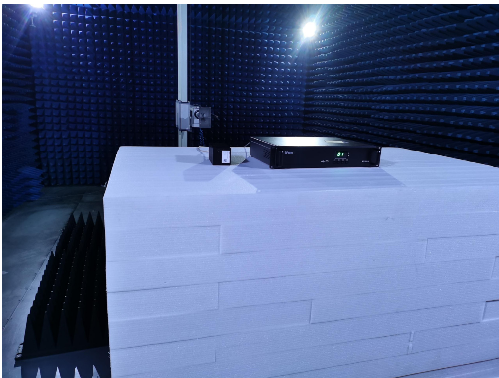
Photo of Radiated Emission Measurement (Above 1G)
