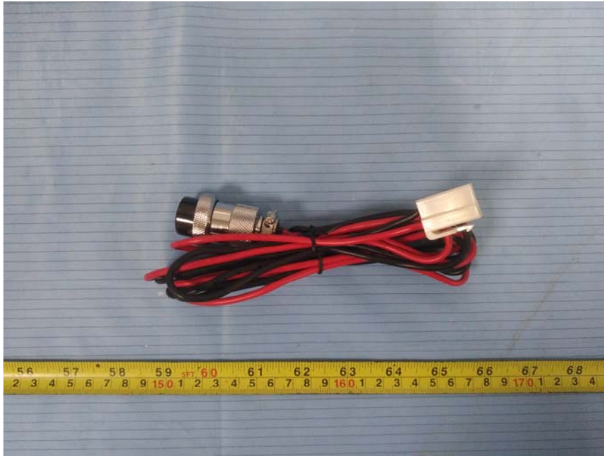
EUT – DC Cable View
