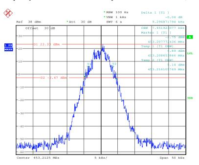
Frequency 453.2125 MHz: 99% Occupied & 26 dB Bandwidth, Low Power
