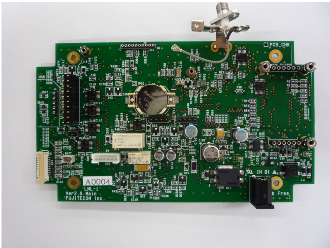
View of main PCB without RF module and SD card module
