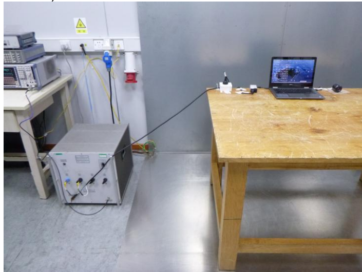
Radiated Emissions (30MHz-1GHz)
