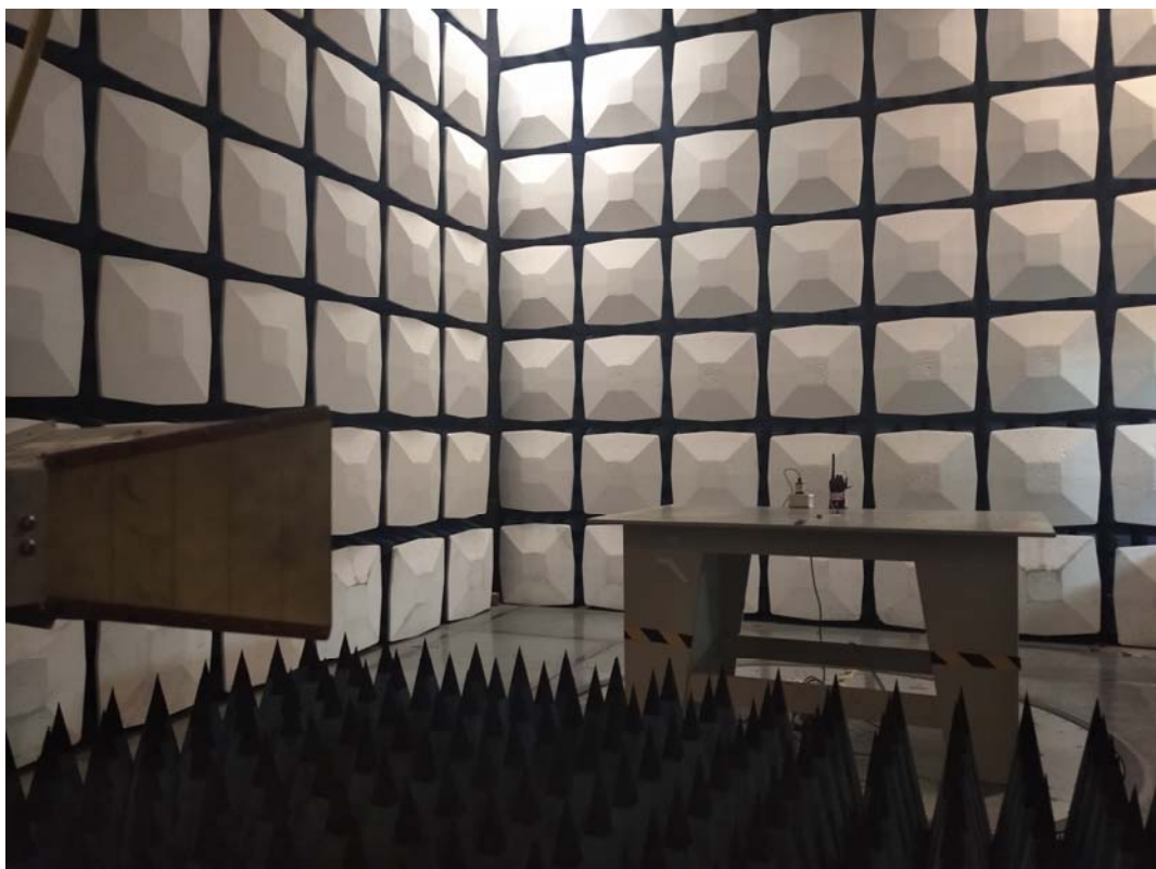
Radiated Emission Above 1GHz Rear View
