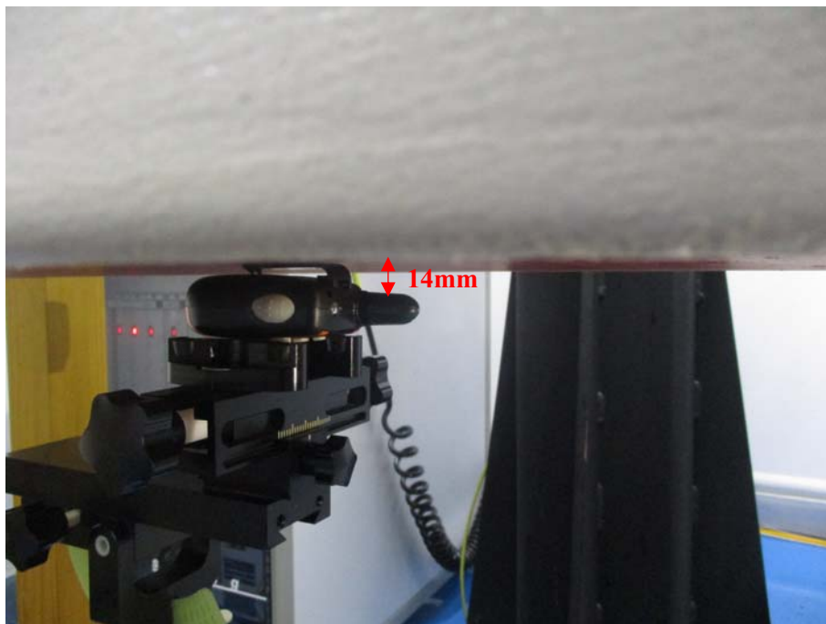
Body Worn Back Setup Photo(0mm)
