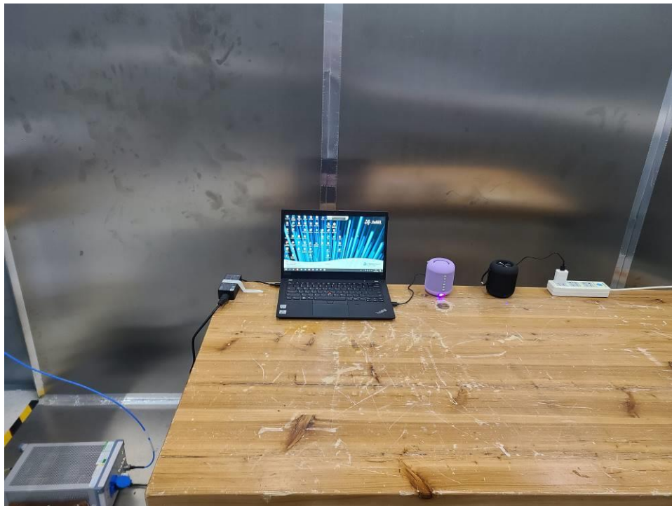
Photograph 3: Set-up for Conducted Emission on AC Mains
