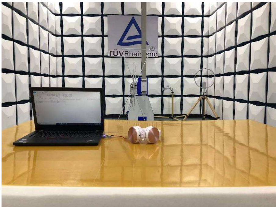
Photograph 2: Set-up for Radiated Spurious Emission, 30MHz ~ 1GHz
