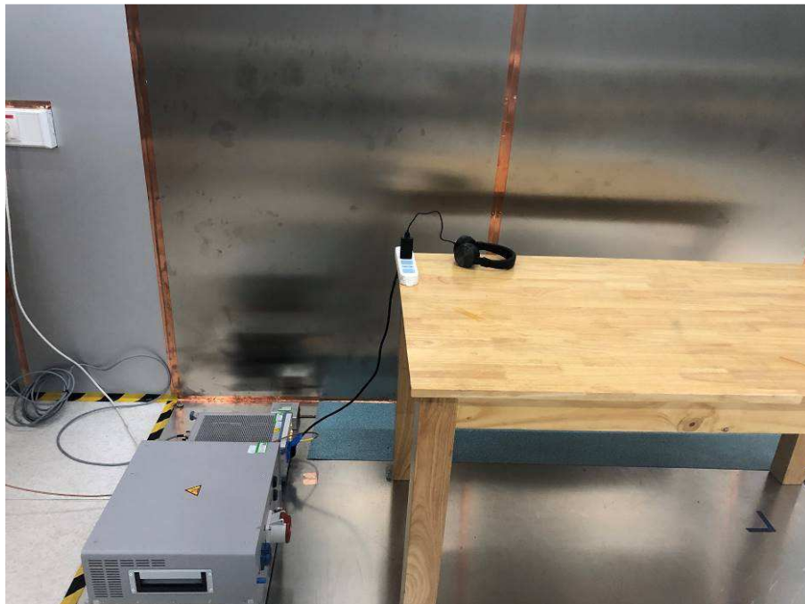
Photograph 4: Set-up for Conducted Emission on AC Mains
