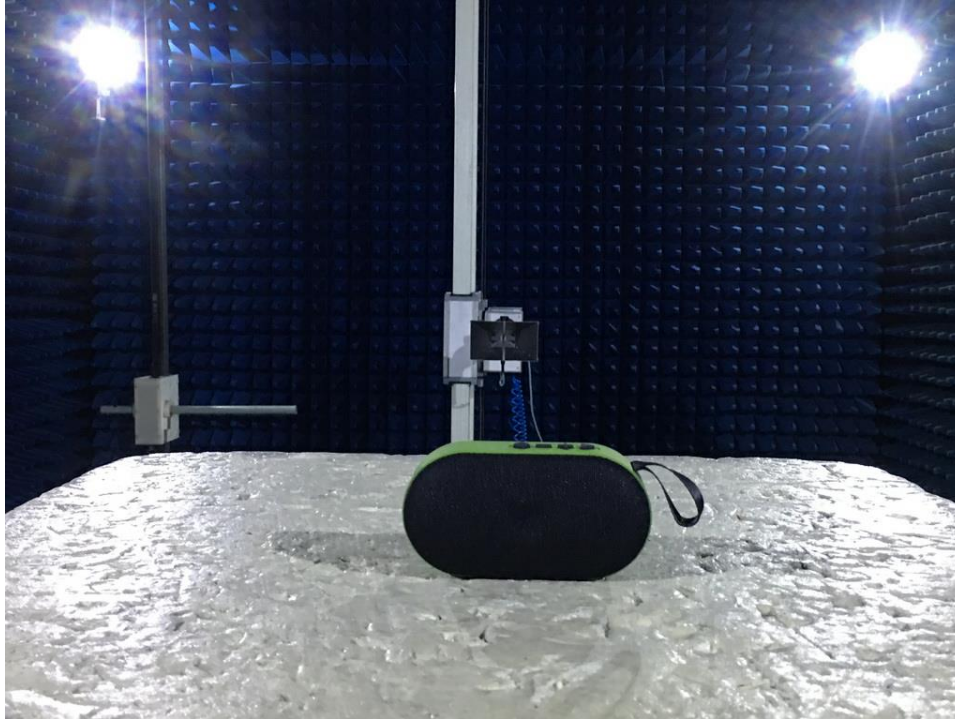
Photograph 3: Set-up for Spurious Emissions (1GHz-18GHz)
