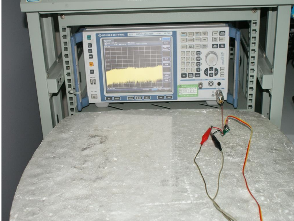
Photograph 5: Set-up for Radio Spetrum test
