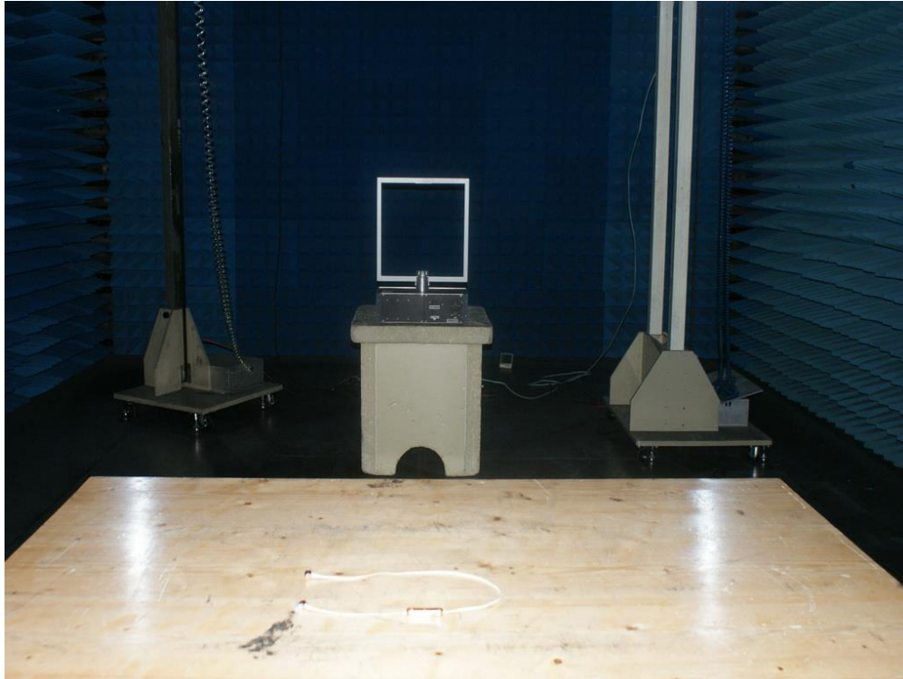
Photograph 2: Set-up for Spurious Emissions (30MHz-1GHz)
