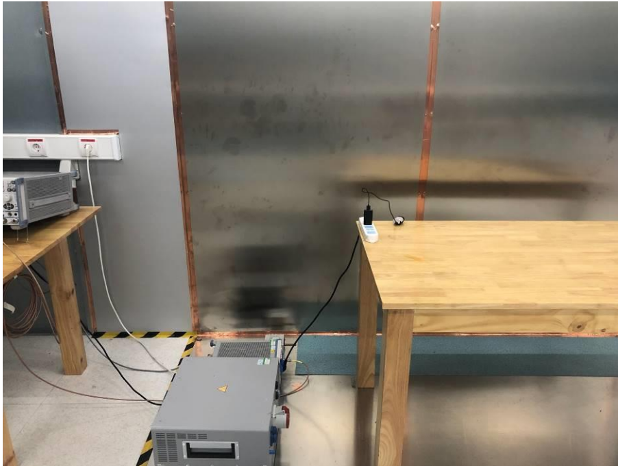
Photograph 3: Set-up for Conducted Emission on AC Mains
