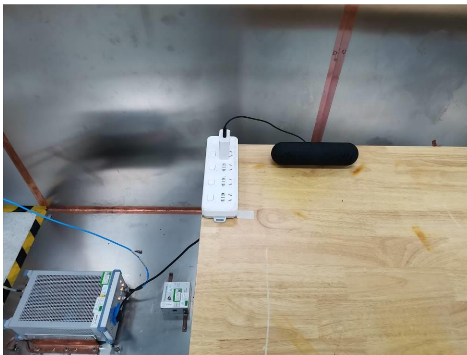
Photograph 1: Set-up for Conducted Emission on AC Mains
