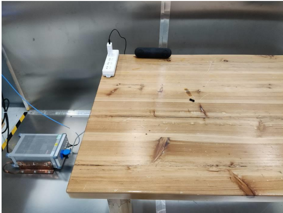
Photograph 1: Set-up for Conducted Emission on AC Mains
