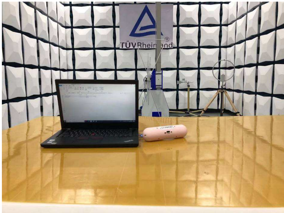
Photograph 2: Set-up for Radiated Spurious Emission, 30MHz ~ 1GHz
