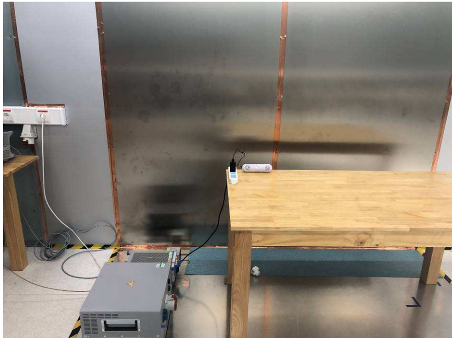
Photograph 4: Set-up for Conducted Emission on AC Mains
